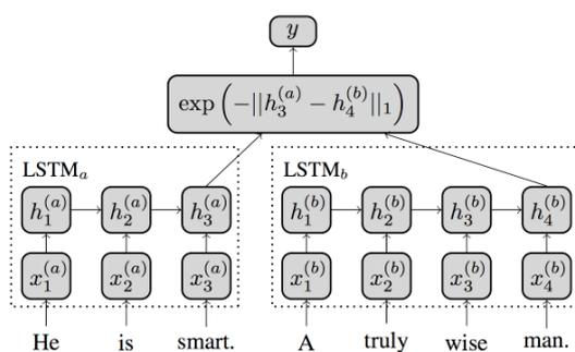
Figure: Siamese LSTM Model Architecture
