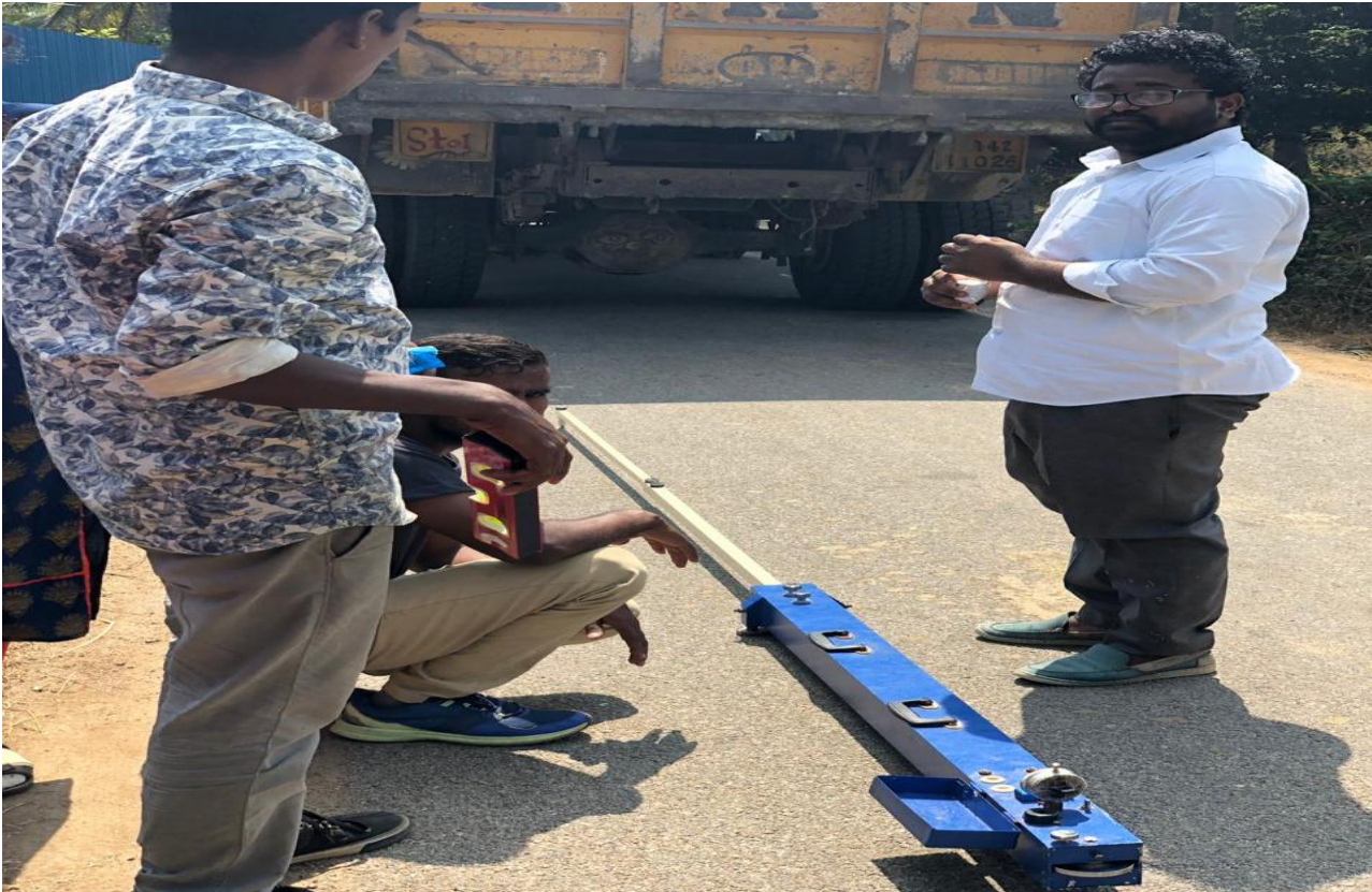
Fig -5: CARRYING OUT BBD TEST
