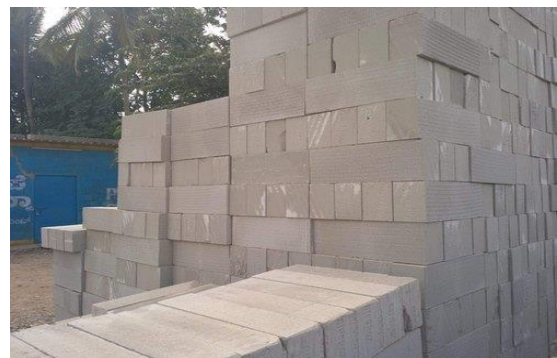
Fig. No. 2.1.1 AAC Blocks (From Actual Site)
