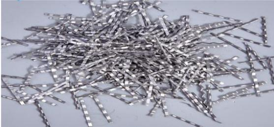
**Fig 3: Steel fibre**
