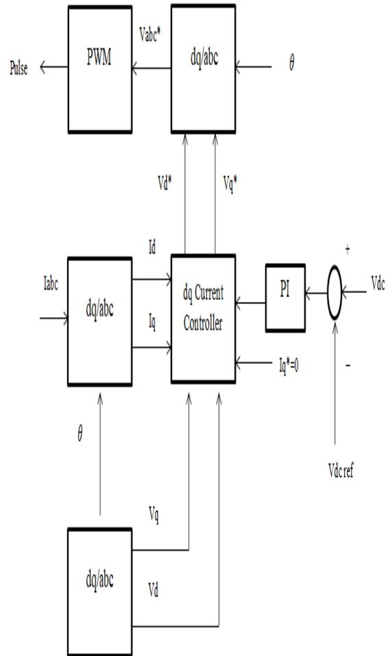
Figure 3 Control Scheme of VSC.
