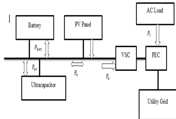
Figure 1 DC micro-grid system layout.
