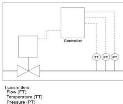
Fig 5. Final control element
