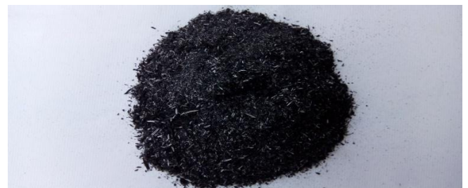
Figure: Collection and Purification of Rice Straw Ash at Site
