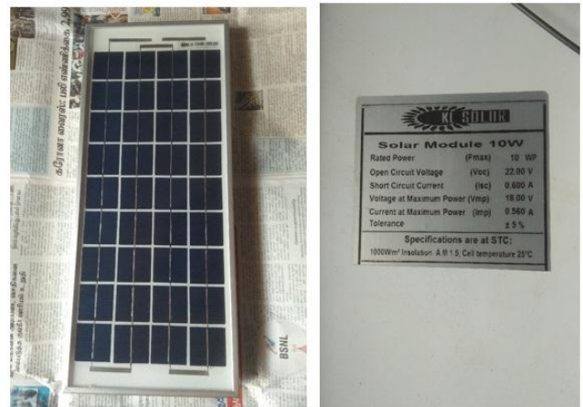
Fig 7. Photograph of Solar Panel
