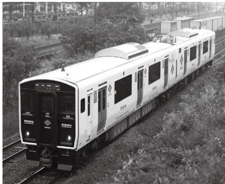
Figure.1 Series BEC819 Battery-Powered Train Charged From AC Overhead Line. High-Capacity Li-Ion Batteries (About 360 Kwh Output) Are Installed Under The Floor Of The Train.
