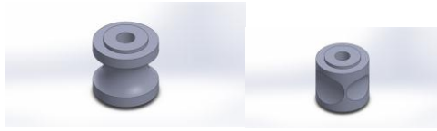
Fig-6 (a)Die with single groove (b)Die with multiple grooves of different sizes
