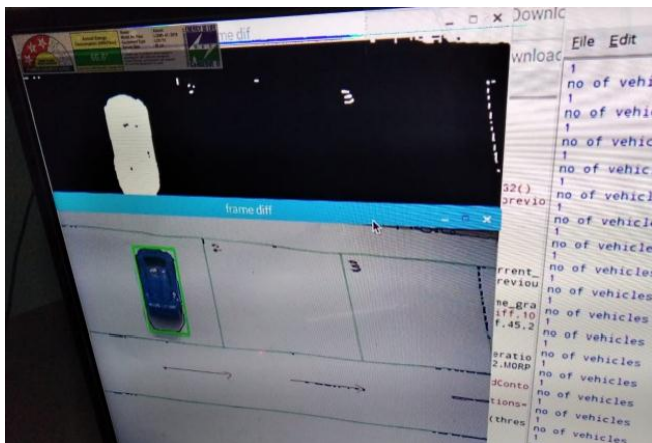
Fig. 9 background subtraction showing single slot occupied
