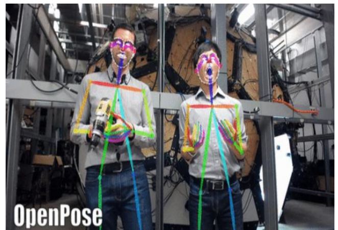
Fig.4 : Real-time multi-person system to jointly detect human body, hand, facial, and foot keypoints (in total 135 keypoints) on single images[1].
