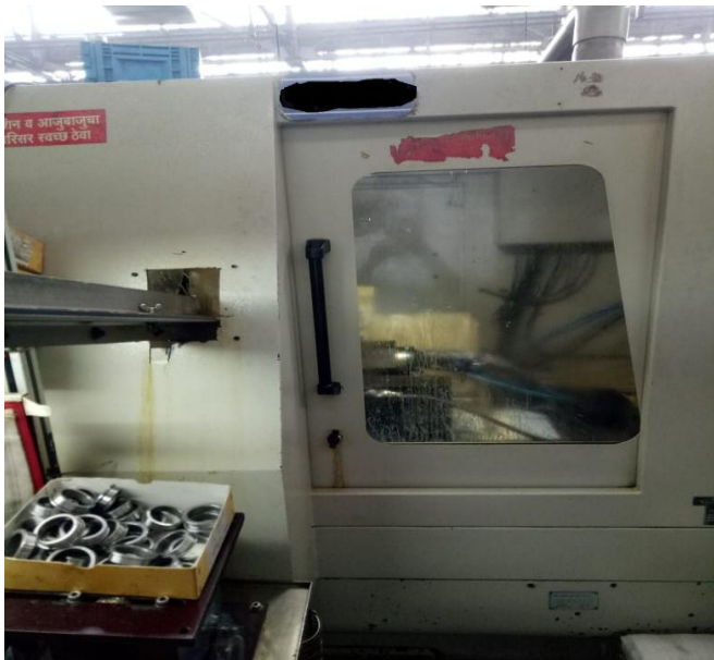
Figure 2.1: CIMAT 1F-CE CNC machine
