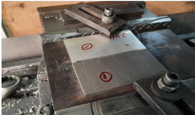
Figure 2.7 plates are placed on milling machine flat and hard tight the clamps, advancing side 2014& 6082 retreating side
