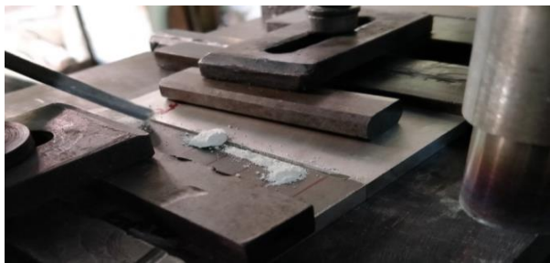
Powder inserting in groove between both plates
