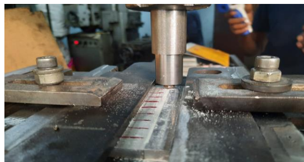
Tool mounting on joint of both plates edges
