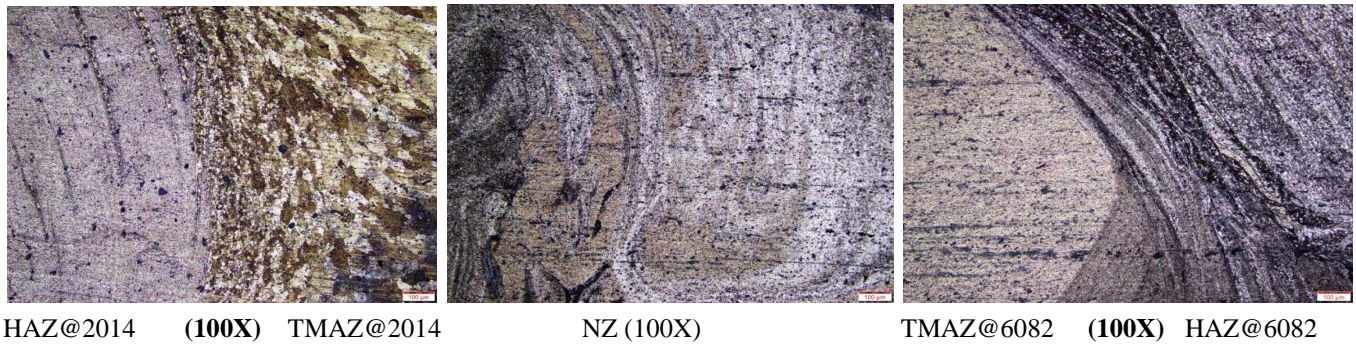
Figure 3.7 Microstructure of Welded Specimen No: 04 at 1120rpm; 25 mm/min weld speed; 1.5 tilt angles
