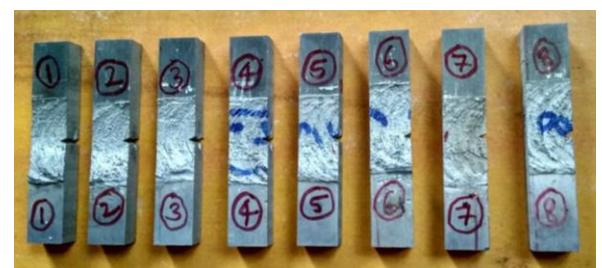
Figure 2.13: Izod impact test samples after EDM wire cut based on ASTM D256
