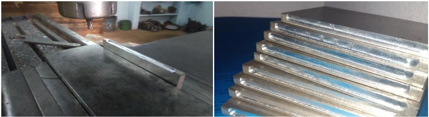
Figure 2.3 work pieces after cutting the groove
