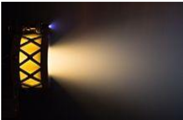
Fig-4 Busek's BIT-3 ion thruster proposed for NASA's Lunar IceCube mission
