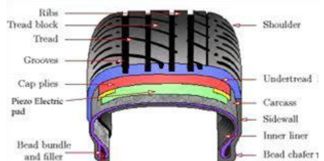
Fig -7: Piezoelectric tire installed with PZT pad [17]
