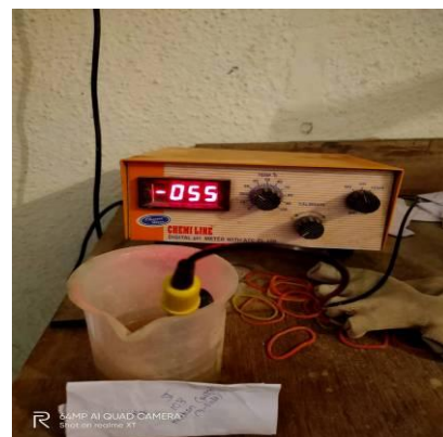
Fig -10 Testing of pH of concrete sample
