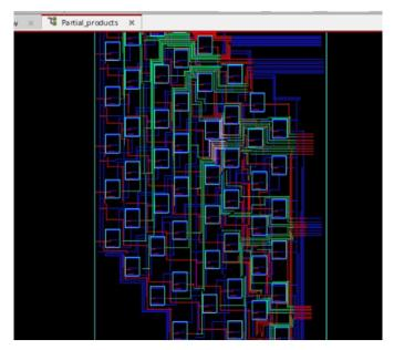
Fig-8: Layout of Partial Product design
