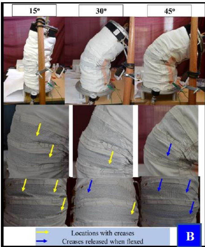
Fig - 5: Pressurized module. Arrows point to creases in the knee area
