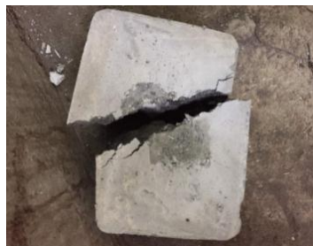
Fig 6.9: Ultimately failed specimen
