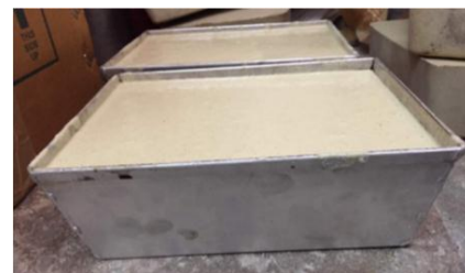
Fig 5.2: Impact testing specimen with mold
