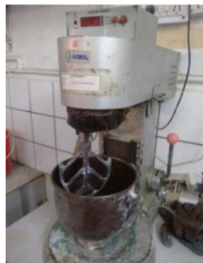
Fig 7.2: Stirrer and vessel used for large batch mixing of polycrete
