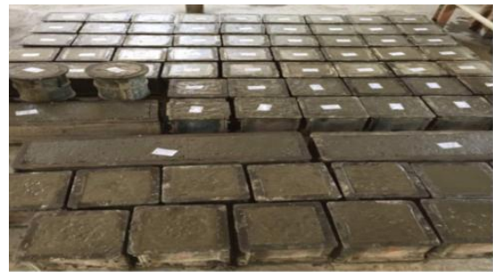
Fig 5.1: Casted concrete compression and flexural specimens
