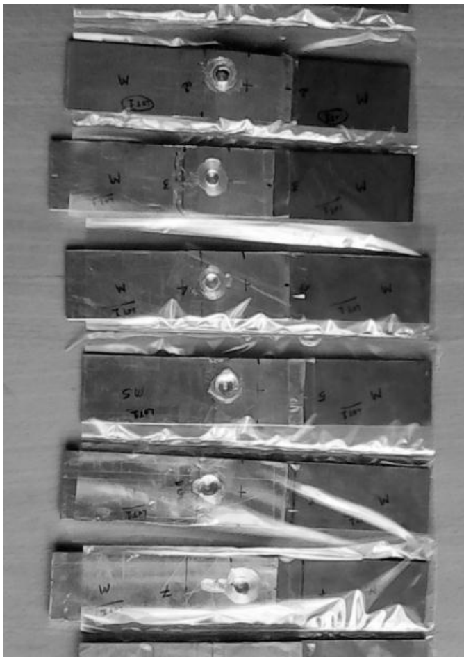
Fig -3. Friction Stir Spot Welded Joints
