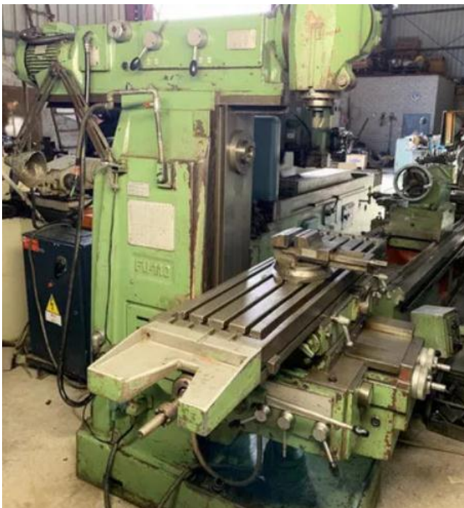
Fig -1. Friction Stir Spot Welding Equipment
