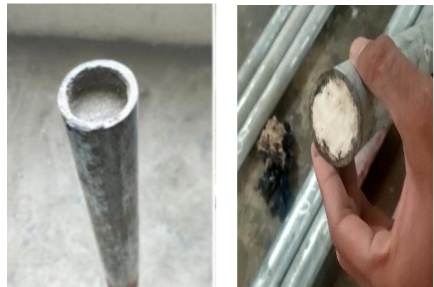
Fig 4.4.1.1 Creating of gap in the specimen to undergo push out test at the base of specimen
