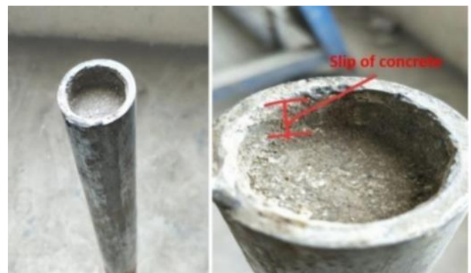
Fig 4.6.4 Specimen after push out test
