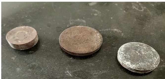
Fig 4.6.2 Solid cylinders used to transfer load only on concrete infill
