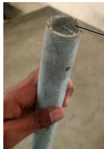
Fig 4.4.3 Specimen after push out test
