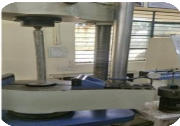
Fig 4.4.1 Loading setup in UTM machine
