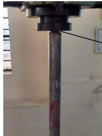
Fig 4.4.2 Solid cylinder arrangement for Load transfer
