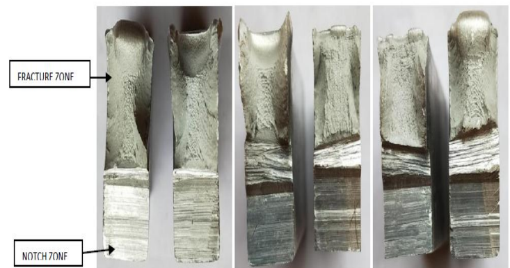
Fig- 3.4 Fractured surface of cryogenic treated specimens
