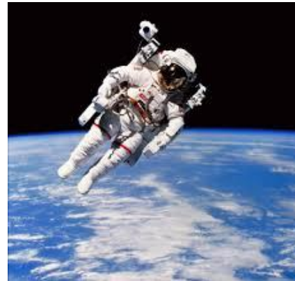
Fig -6.2: Manned Maneuvering Unit from lockheedmartin.com
