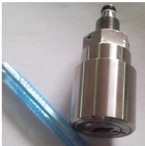
Fig -2.7: Fill/Vent Valve from Researchgate.net
