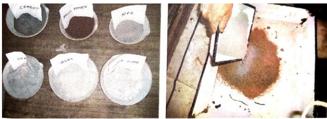
Figure 4.1: Process of Proportioning of the ingredients.
