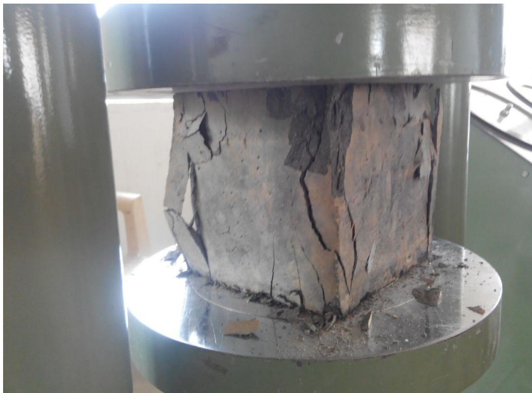
Fig 5.2 Failure of cube specimen
