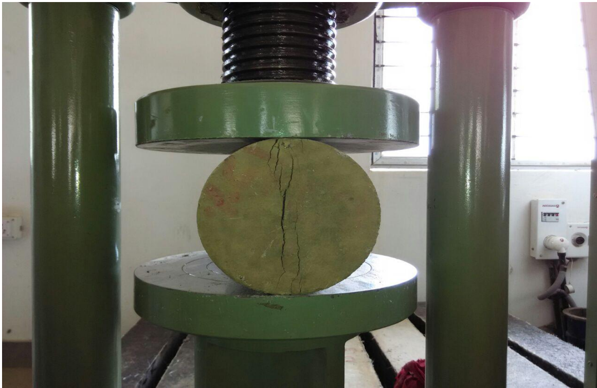
Fig 5.14 Failure of cylinder specimen
