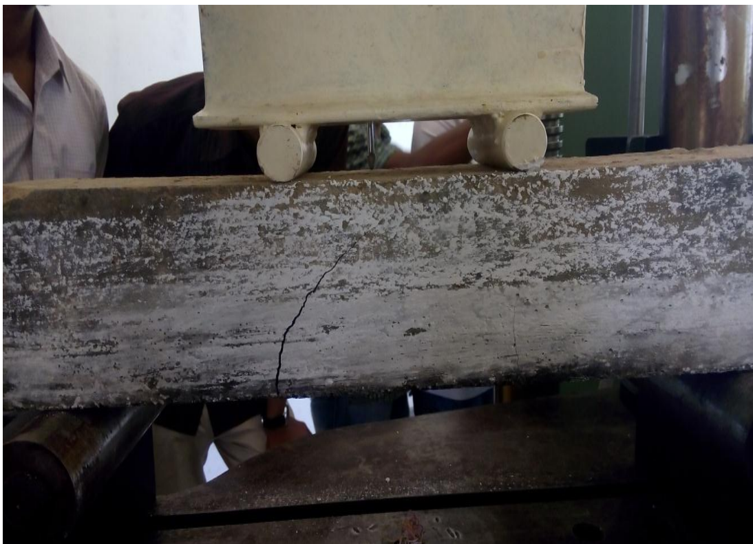
Fig 5.8 Failure of beam specimen
