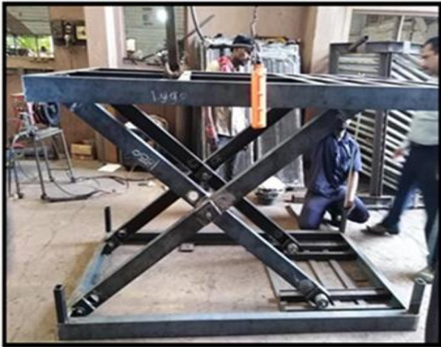
Fig -9: Hydraulic Lift
