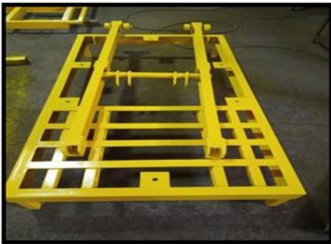
Fig -10: Spray Painted Lifting Structure
