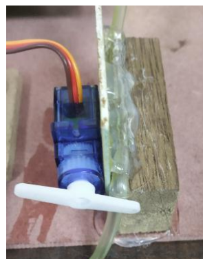
Fig -10: Saline valve blocked
