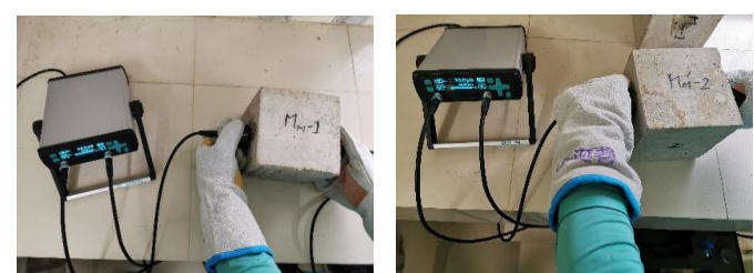
Fig-14: UPV test of the specimens immediately after drying of the specimens for 24 hrs at 105°C.
