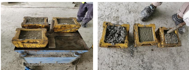
Fig-3: Sample in vibration table for vibro compaction & sample compaction by normal tamping with 16 mm MS bar.
