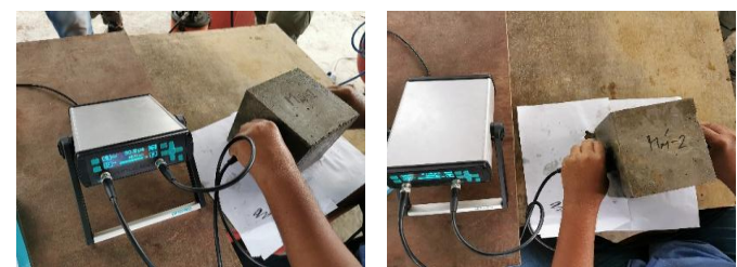
Fig-14: UPV test of the moist specimens immediately after removal from curing tank at 28-days.
