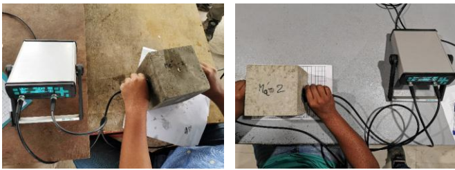
Fig-2: UPV test of samples of different conditioning of curing.
