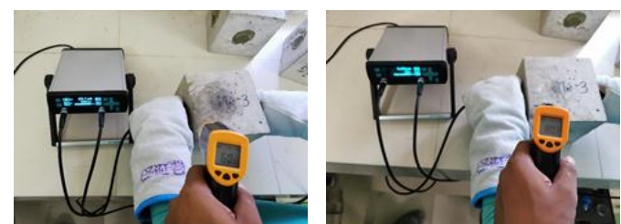
Fig-8: UPV testing & temperature checking.
