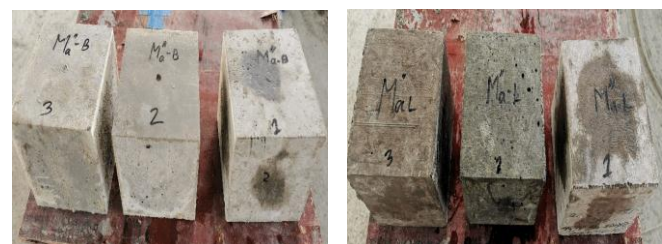
Fig-5: Sample with crushed Basalt stone aggregate (Left) & samples with crushed Lime stone aggregate (Right)
