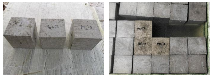
Fig-1: Sample in water tank for curing & sample in exposed sunlight & ambient air condition.
