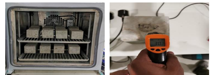
Fig-7: Sample oven for heating (Left) & samples before testing temperature check by thermal scanner (Right)
