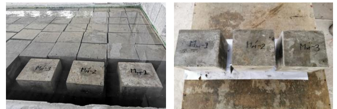
Fig-12: Samples for evaluation of moisture effect in concrete.
