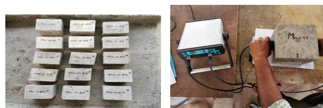
Fig-11: Samples UPV testing of different w/c ratio of concrete.
