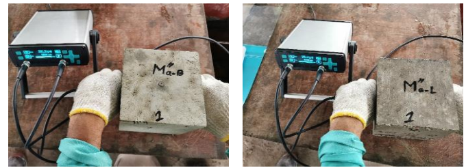
Fig-6: UPV test of samples with different types of coarse aggregate in concrete.
