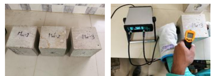
Fig-13: Samples after oven drying at 105°C & UPV test of the specimens after drying at 105°C.
