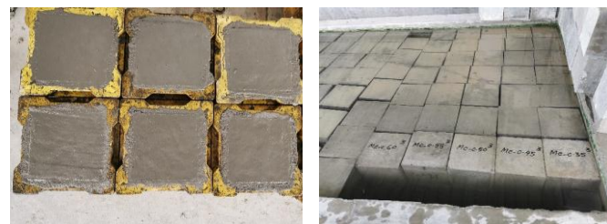
Fig-10: Samples preparation and curing of the specimens.
