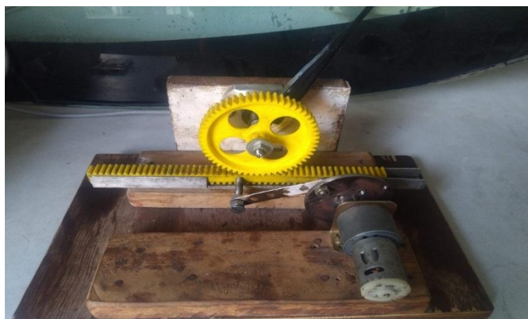
Figure 1: - Electrochemical Rain Sensing (ERS) DC geared Wiper system
