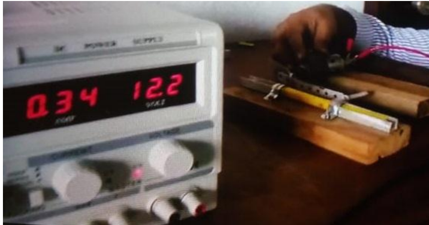
Figure 9-a – Snapshot of video showing voltage and current of ERS wiper system
