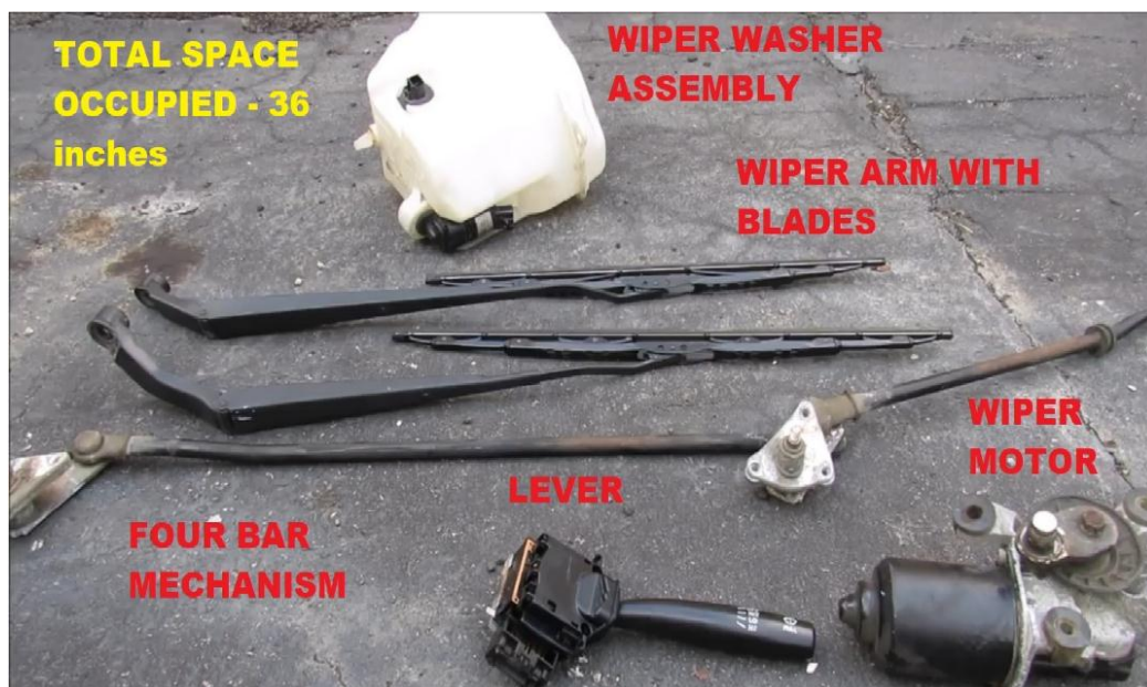
Figure 3 – Various parts of the conventional wiper assembly
