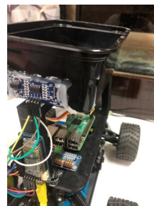
Fig. 2.2.2 Bluetooth beacon and ultrasonic sensor mounted on the delivery robot
