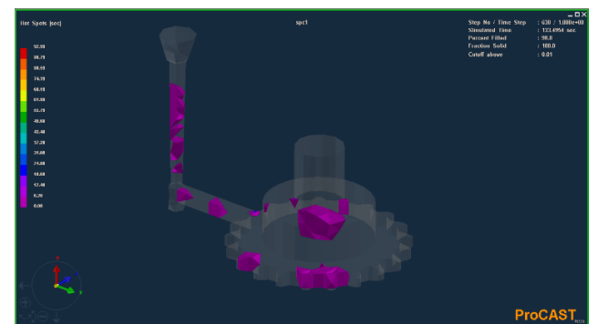
Fig -21: Hotspots in Stainless Steel
