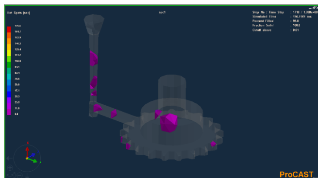
Fig -19: Hotspots in Stainless Steel
