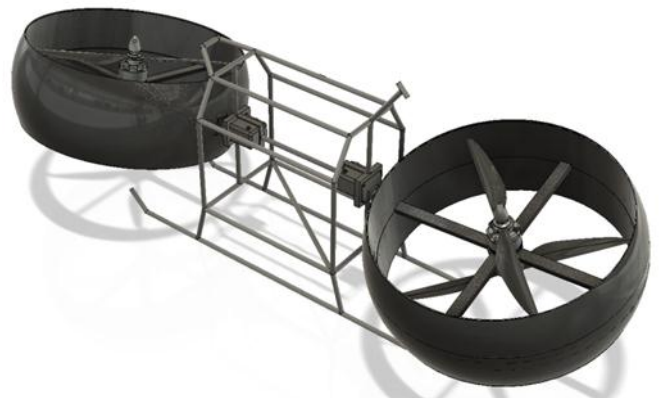
Fig.26: Yaw mechanism- right direction turn
