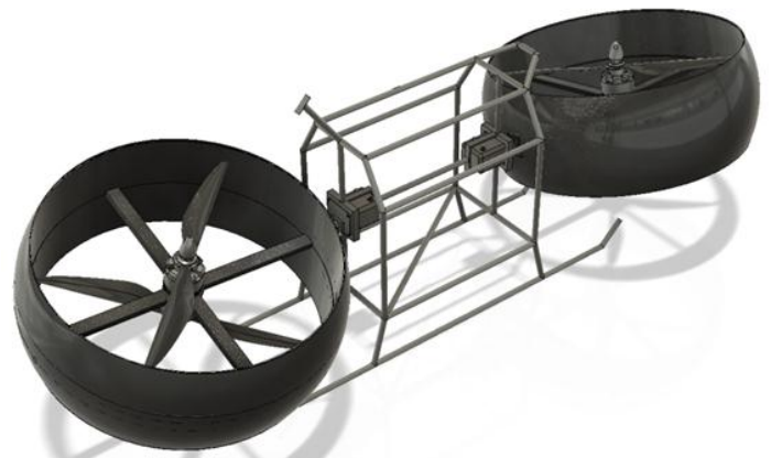
Fig.27: Yaw mechanism- left direction turn
