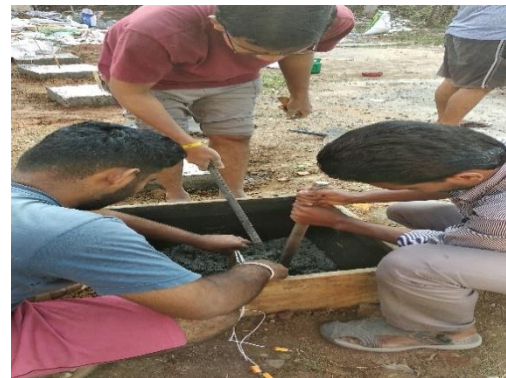
Figure -4: Fixing of thermocouples to wooden bead
