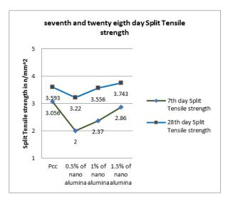
This chapter presents the conclusions reached in experimental work to appreciate the behaviour of Nano-Silica and Nano-Alumina in concrete. M40 mark of concrete was produced with a water-cement ratio of 0.5. The study is limited to appreciate the behaviour of Nano-Silica and Nano-Alumina when added as mineral admixtures to concrete.
