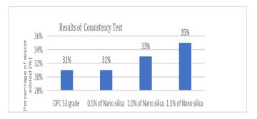
The following graph depicts the results of consistency test carried out on OPC 53 grade cement and Nano-Alumina replaced cement
