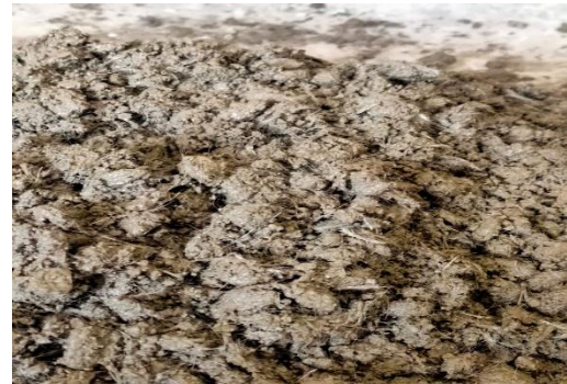
Fig 3: wet mix of Tio 2 and fiber in concrete
