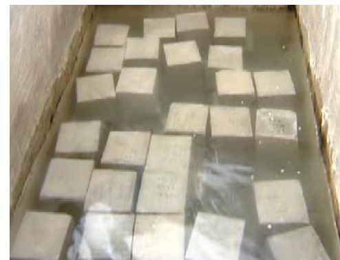
Fig 4: curing of cubes
