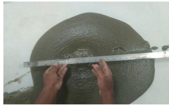
Figure 1: Measuring the slump value in x direction
