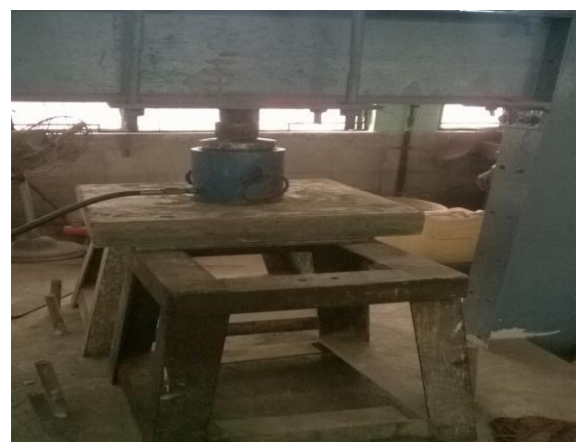
Figure 2: Flexural test on ferro foam panel
