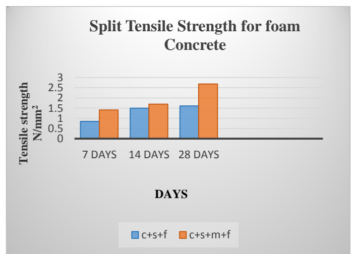
Figure 6: Split tensile strength of foam concrete
