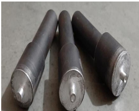
Fig.1 Straight cylindrical probe FSW Tool
