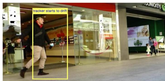
Figure 3.4 The target's auxiliary template may be updated with wrong image content when a tracker starts to drift since much background information is included within the tracker's bounding box.
