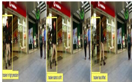
Figure 3.5 When a tracker starts drifting away from the target, it is likely to be stuck at a background object but still recognizes it as the target to track so the auxiliary template is kept updating with some learning rate. Under that case, \text{sim}(F_t^i, F_t^j) will retain high value and keep increasing until it saturates to a rather high value.
