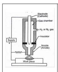
Machining takes place with the help of plasma is called plasma machining. A tungsten electrode acts as negative is enclosed in a chamber, in which inert gas like helium or argon supplied and pass through nozzle. The workpiece is given positive terminal. When supply is given, an arc is formed between electrode and workpiece and the temperature is about 1200 degree Celsius. This temperature ionize the gas and it becomes plasma. As this plasma is directed on workpiece, machining is done.
