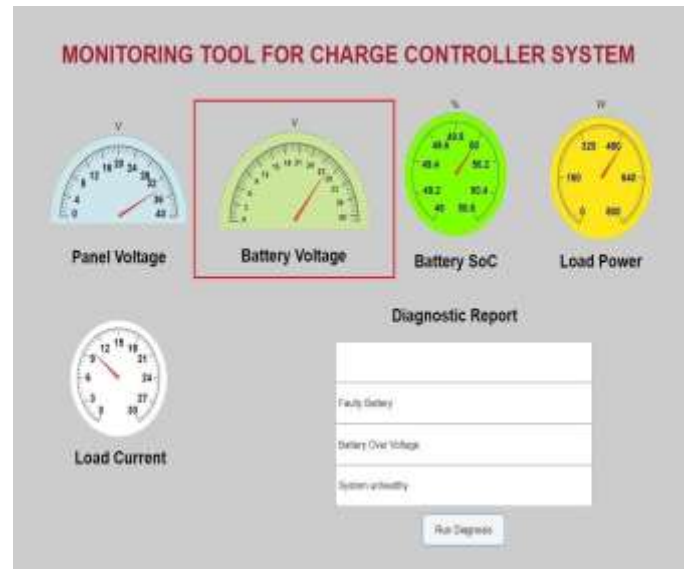
Fig - 6: GUI output for Battery Overvoltage Fault
