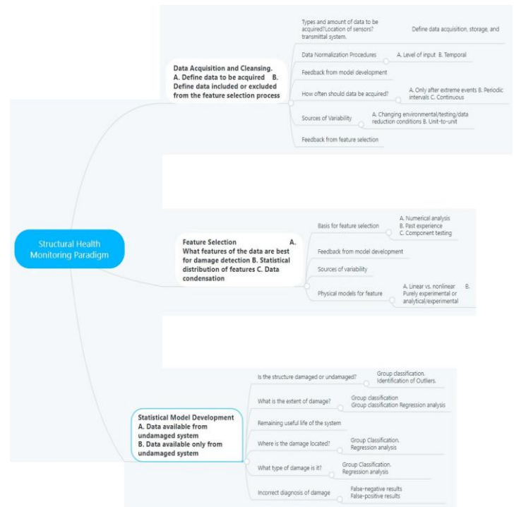
Figure 3: Structural health monitoring paradigm [10]
