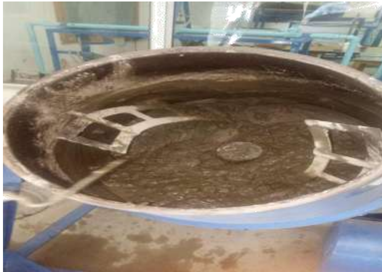
Fig (2.4) Mixer making M20 Grade
