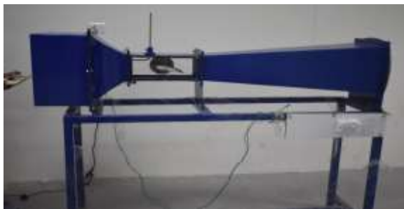
Figure 4.3: Final Assembly of Wind Tunnel
