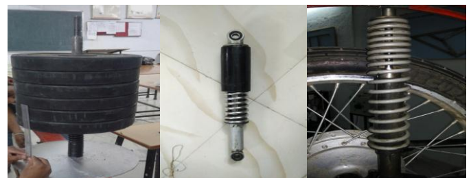
Fig-4: Spring Stiffness Measurement of Splendor Suspension and Honda Shine Suspension
