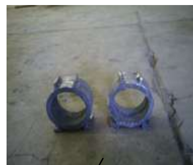
i) After sand removal by hand grinding
