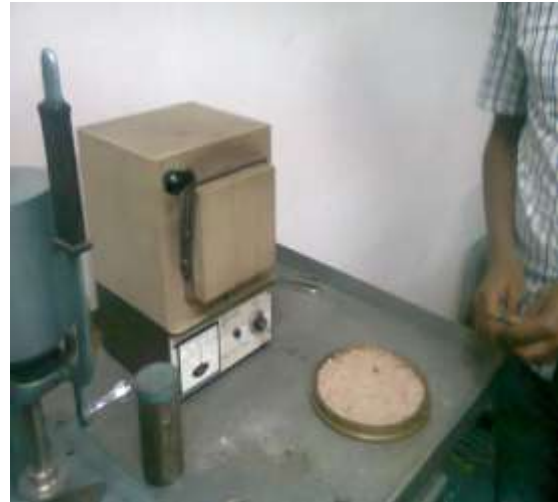
Figure.6 Photo during silica sand drying using oven drier after clay washing
