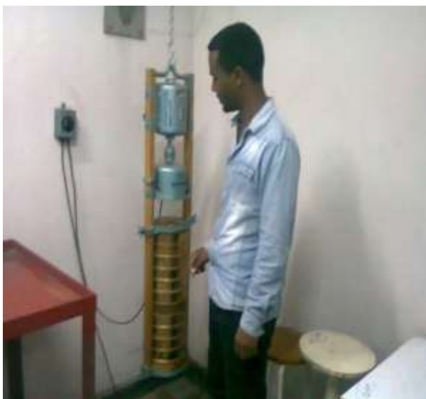
Figure.8 Photo during shaking of sand in sieve shaker and weighing of each sieve with grains on it.
