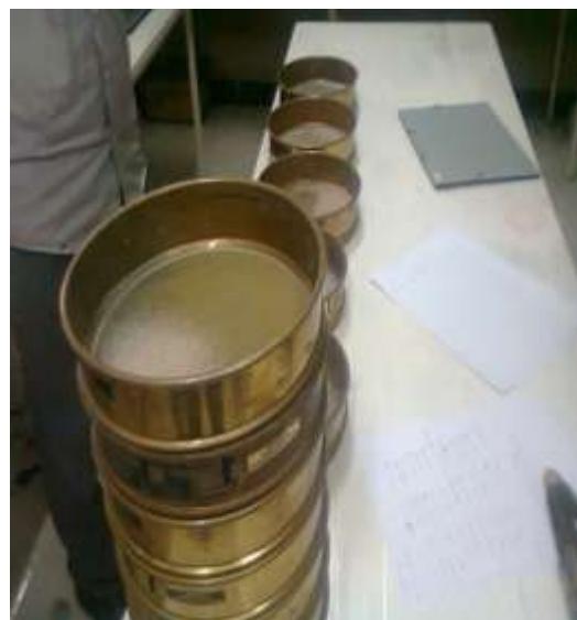
Figure.8 Photo during shaking of sand in sieve shaker and weighing of each sieve with grains on it.
