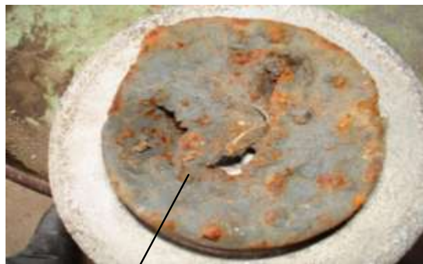
b) Shrinkage due to over melt
