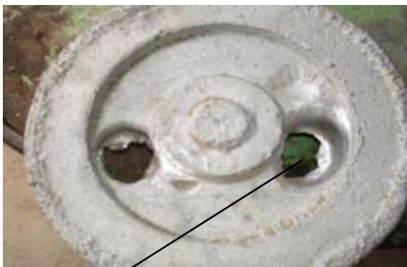
a) Shrinkage due to fast solidification at thin section
