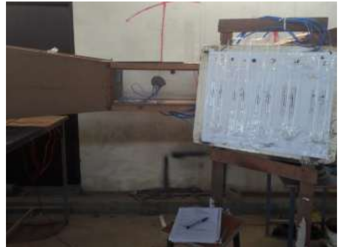
Figure 4. Taking reading in Wind Tunnel
