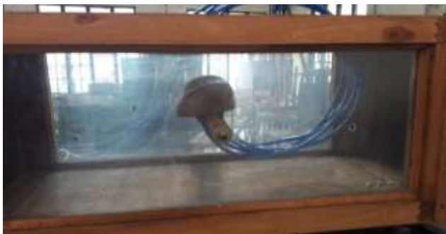
Figure 8. Spherical Helmet in Test Chamber
