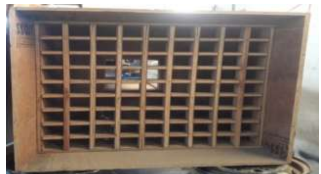
Figure 5. Honeycomb and Screens
