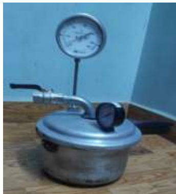
Fig -2: Pyrolysis reactor
