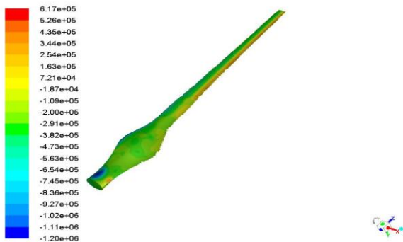
Figure 23: Pressure Side Pressure Contour at \alpha = -5^\circ
