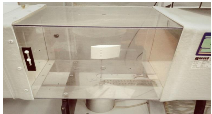
Figure 33: Dimpled S830 Model with Dimples config. #II in Test Section
